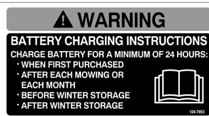
1. Warning—read the *Operator's Manual* for information on charging the battery; contains lead; do not discard.
