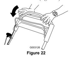
**Important:** When you release the blade control bar, the blade should stop within 3 seconds. If it does not stop properly, stop using your mower immediately and contact an Authorized Service Dealer.
