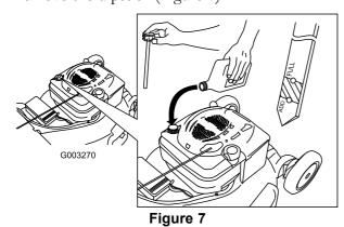
2. **Slowly** pour oil into the oil fill tube until the oil level reaches the Full line on the dipstick (Figure 7). **Do not overfill.** (Max. fill: 20 oz. (0.59 l), type: SAE 30W detergent oil with an API service classification of SF, SG, SH, SJ, SL, or higher.)
