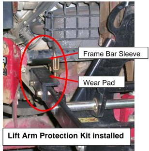
If the rear QAS attachments (Tooth Rake, Rear Broom or Drag Mat Carrier) already have the plastic Wear Pad on the Lift Arm, then no additional action would be required.
