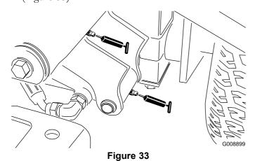
• Right front lift arm pivot and lift cylinder (2) (Figure 34)
