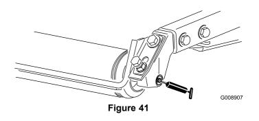
**Note:** The flush fittings on the rollers (Figure 27) require a grease gun nozzle adapter. Order Toro Part No. 107-1998 from your Authorized Toro Distributor.
