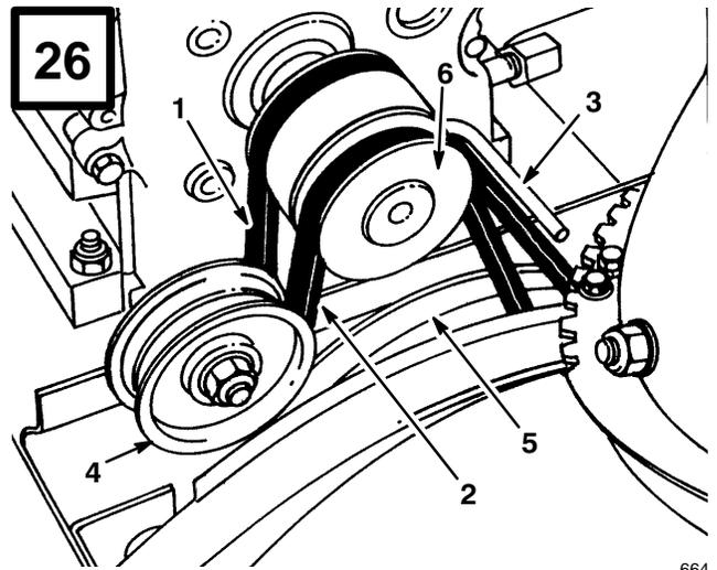
1. Traction drive belt                      5. Large auger/impeller pulley
