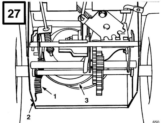
1. Spring                                              3. Large traction pulley
