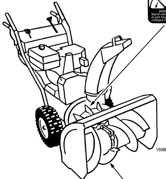
**LOW SPEED AUGER HAS MOVING PINCH POINT, CLOSE TO OPENING.**
