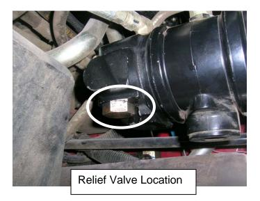
Units produced with serial numbers higher than listed already have Relief Valve (115-8032) installed.
