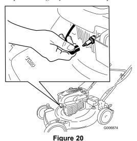
3. After performing the maintenance procedure(s), connect the spark plug wire to the spark plug.
