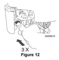
**Note:** If the air temperature is below 55°F (13°C), firmly push the primer in 5 times.
