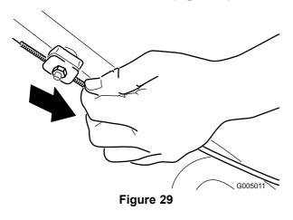
3. Tighten the nut on the cable support.
