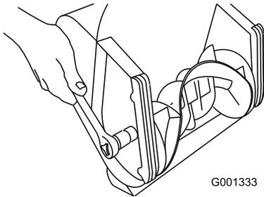
2. Remove the old rotor from the housing.
