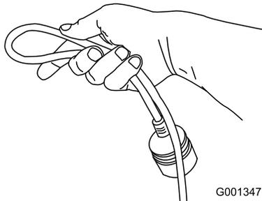
2. Insert the loop through the hole in the back of the upper handle, securing the loop around the hook.
