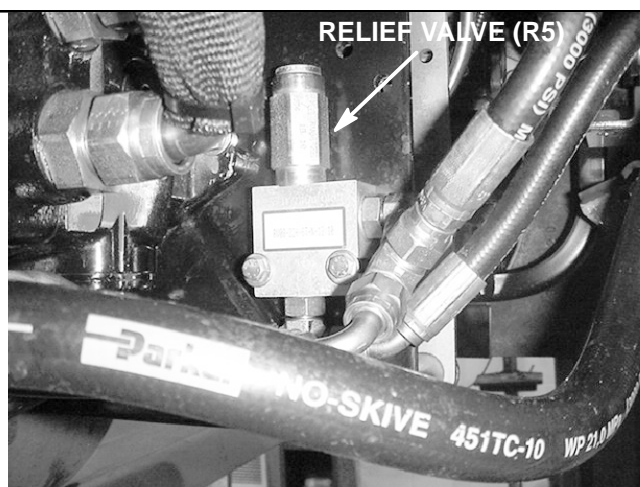
PHOTO SHOWS RELIEF VALVE (R5) AS USED IN MACHINES WITH SERIAL NUMBER UNDER 220999999
