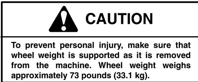
B. Carefully slide wheel weight from weight studs.
