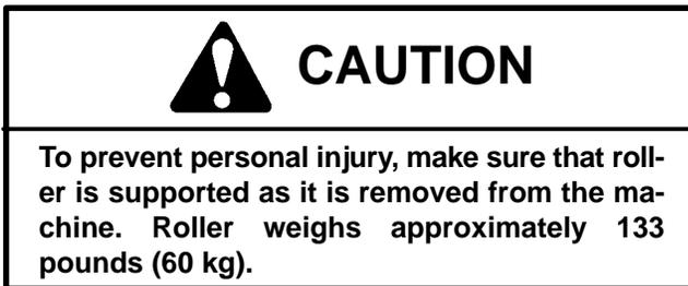
6. Remove roller with flange bearings from under machine.
