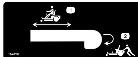
1. Bypass lever position for operating the machine
