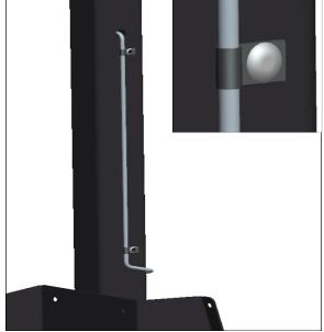
3. Drill out existing rivets (2xLeft & 2xRight) on the 2-Post. Retain vent tubes and tube clamps.
