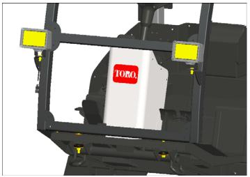
11. Install flashers (LH and RH Side) on provided flasher brackets (welded to 2-Post ROPS Extension). Use retained hardware.
