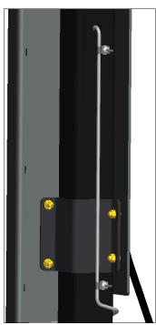
13. Install vent tube (RH and LH Side). Use spacer, rivet no. 88 (included in parts box) and the retained vent tube clamps.
