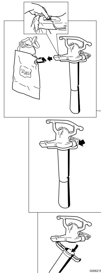
2. Install the blower tube and then the inlet cover onto the blower housing.
