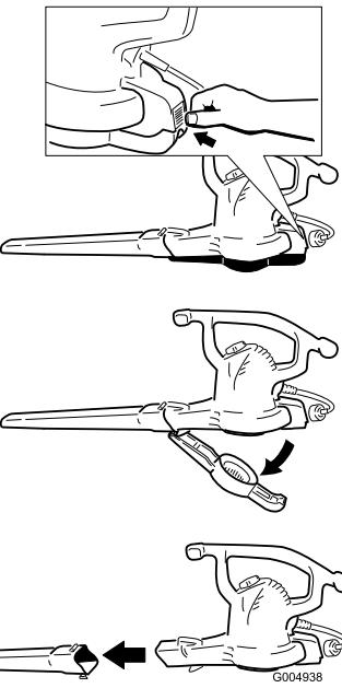
2. Install the vacuum tube onto the blower housing.
