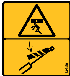
93-9899: Crush hazard Install the cylinder lock when extended
