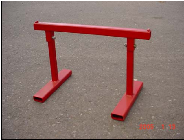
Figure 29: Cross conveyor storage stands
