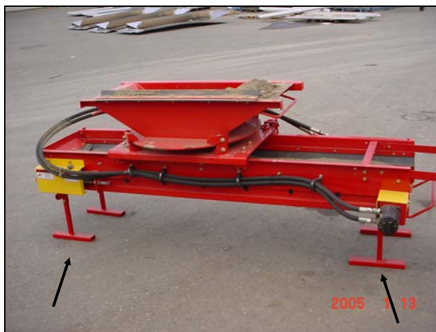
Figure 27: Cross conveyor on storage stands
