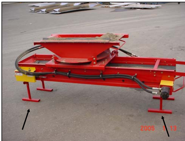
Figure 27: Cross conveyor on storage stands
