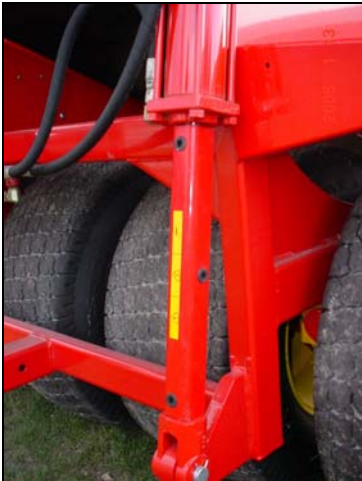
Figure 6: Hydraulic cylinder support in place
