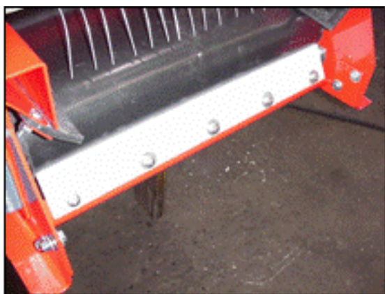
Figure 23: Belt cleaning scraper assembly
