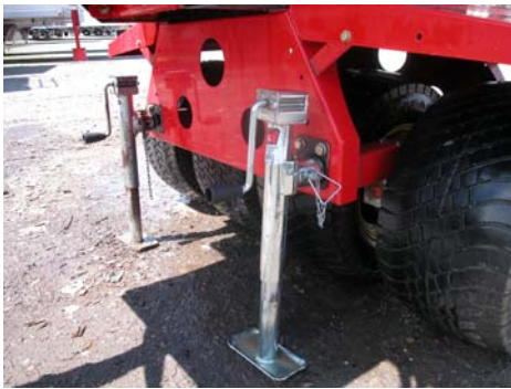
Figure 4: Jack stands On Truckster Direct Connect
