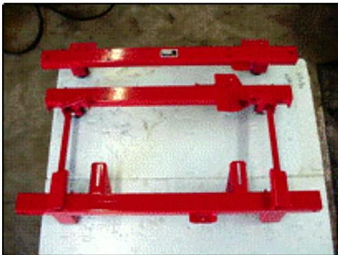
**Figure 24: Installing center cross member**
