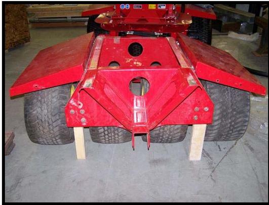
**Figure 14: Fenders Installed**
