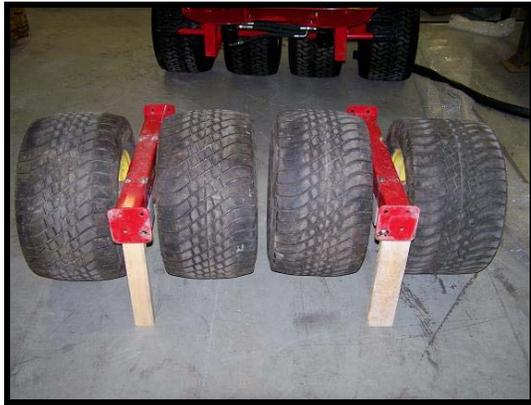
**Figure 10: Blocked Suspension Tubes**
