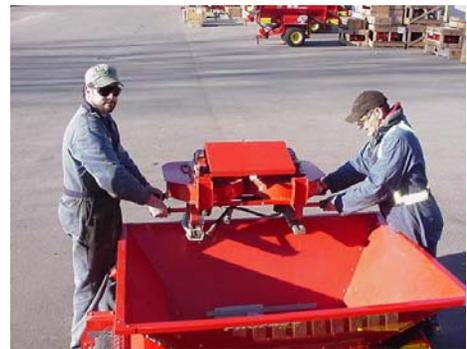
**Figure 3: Removing Twin Spinner from hopper**
