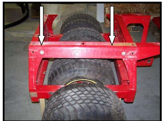
**Figure 13: Only Use Inner Bolt Holes**
