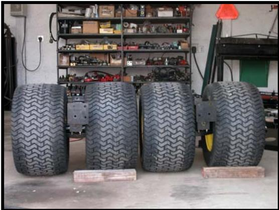
**Figure 52: Block Suspension**
