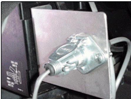
**Figure 59: Mounting electrical plug bracket**
