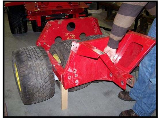
**Figure 12: Install Front Brace**
