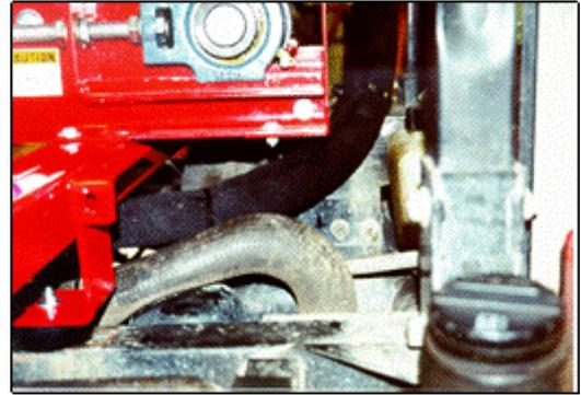
**Figure 35: Route hydraulic hose away from other components**
