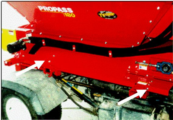
**Figure 31: Installing Button head bolts**
