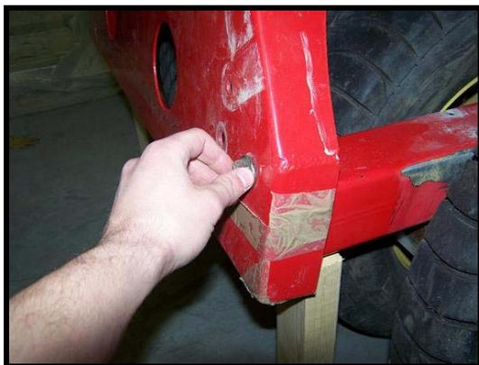
**Figure 11: Finger Tighten Bolts**
