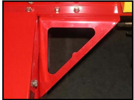
**Figure 16: Left Side Gusset Has Dimple**
