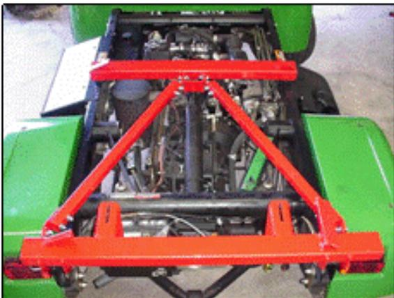
**Figure 43: Installing braces on center cross member**
