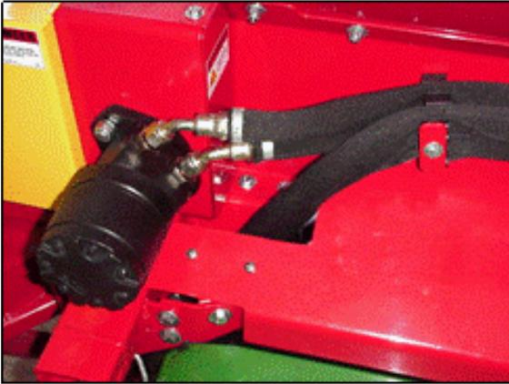
**Figure 49: Routing Twin Spinner hoses**
