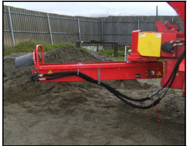
**Figure 70: Conveyor hose routing**
