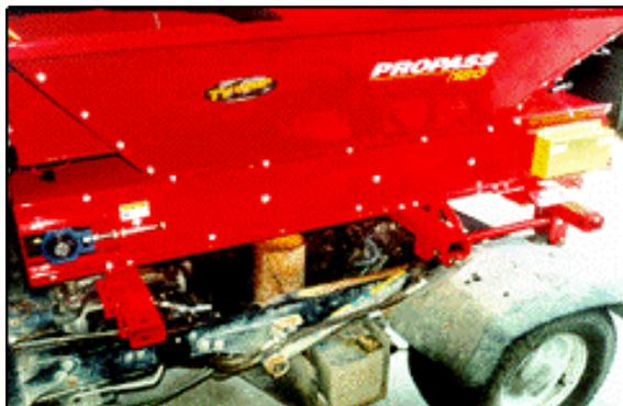
**Figure 28: Lowering ProPass onto Workman**
