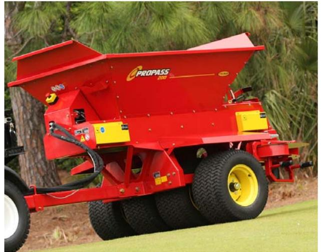
**Figure 63: Hopper extension kit installed**
