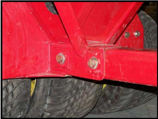
**Figure 18: Hitch Installed**
