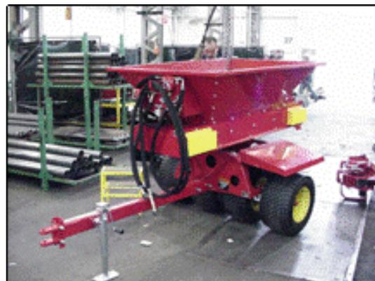
**Figure 8: Lowering ProPass onto chassis**
