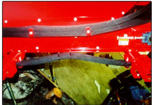
**Figure 36: Ensure proper tension of hydraulic hoses**
