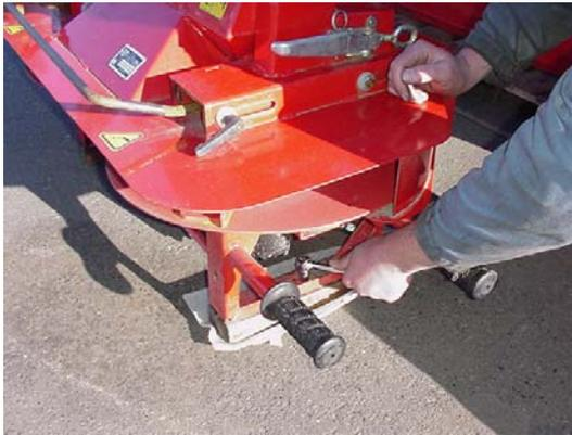
**Figure 5: Removing packing studs and foam**
