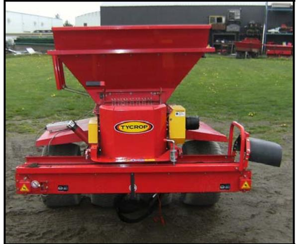
**Figure 69: Conveyor pinned in the travel position**
