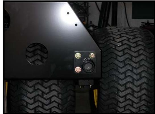
**Figure 53: Jack Mount Installed**
