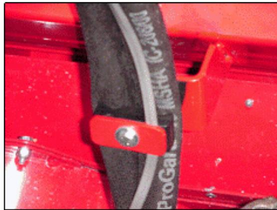
**Figure 51: Attaching hydraulic hoses**
