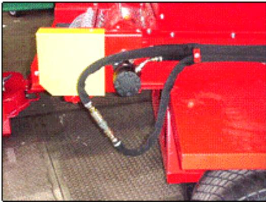
**Figure 9: Connecting quick couplers**
