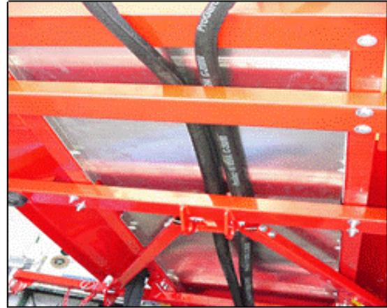
**Figure 50: Routing hydraulic hoses**
