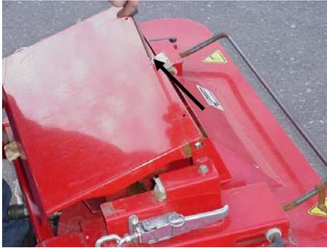
**Figure 4: Removing wood from Twin Spinner guard**
