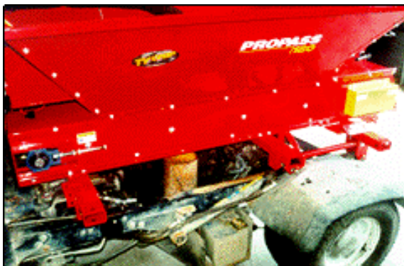
Figure 28: Lowering ProPass onto Workman
