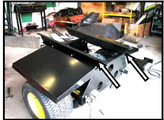
Figure 57: Side Rails Installed
