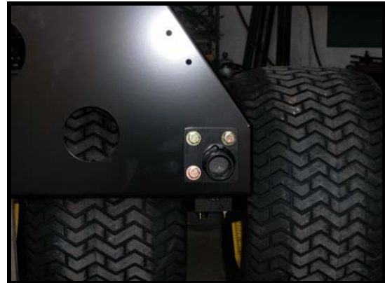
Figure 53: Jack Mount Installed
