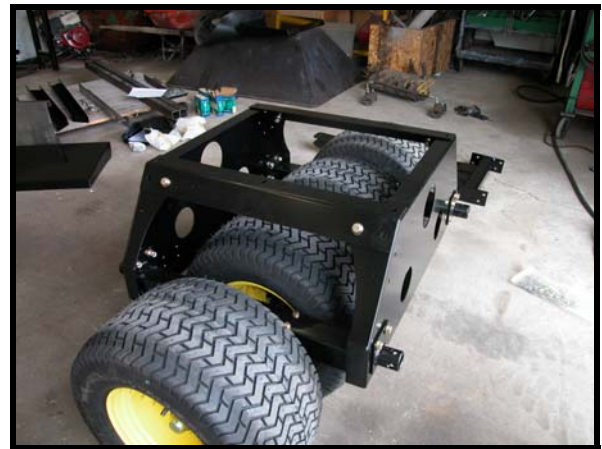
Figure 54: Cross Members Installed
