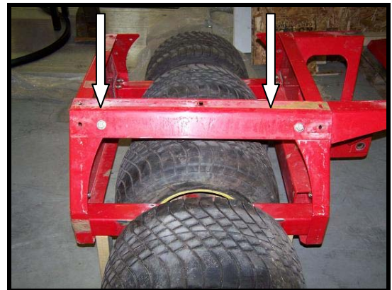
Figure 13: Only Use Inner Bolt Holes
