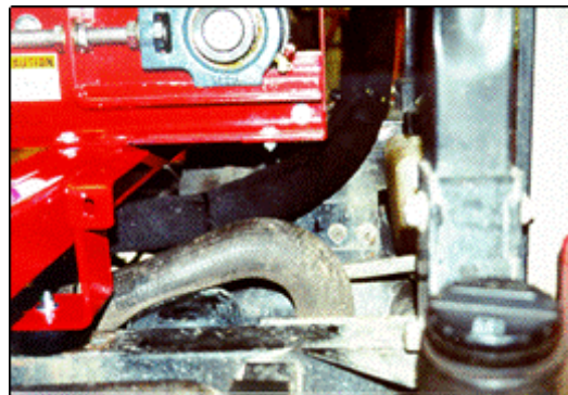
Figure 35: Route hydraulic hose away from other components
