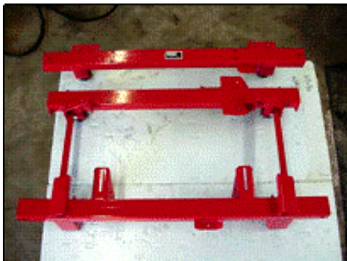
Figure 24: Installing center cross member
