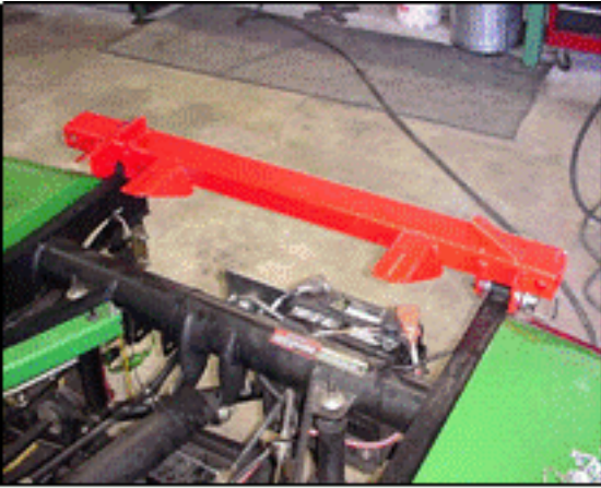
Figure 37: Installing rear cross member
