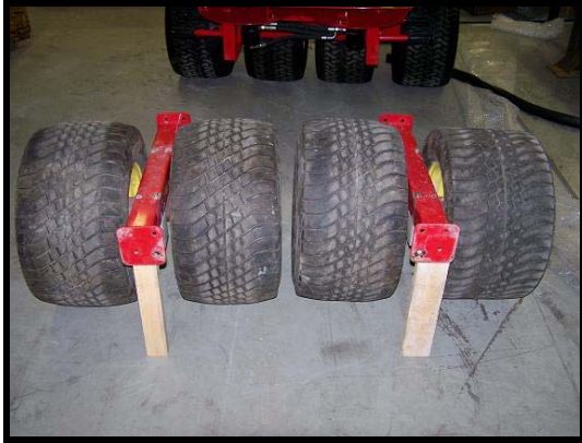
Figure 10: Blocked Suspension Tubes
