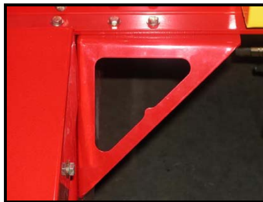
Figure 16: Left Side Gusset Has Dimple
