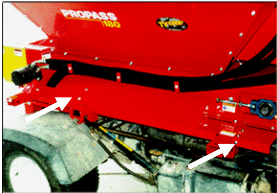
Figure 31: Installing Button head bolts
