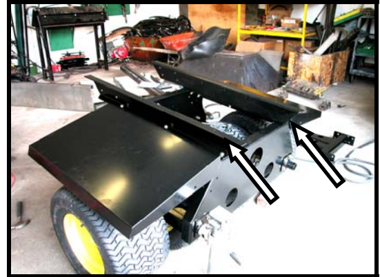
Figure 57: Side Rails Installed
