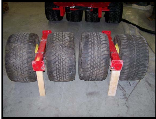
Figure 10: Blocked Suspension Tubes
