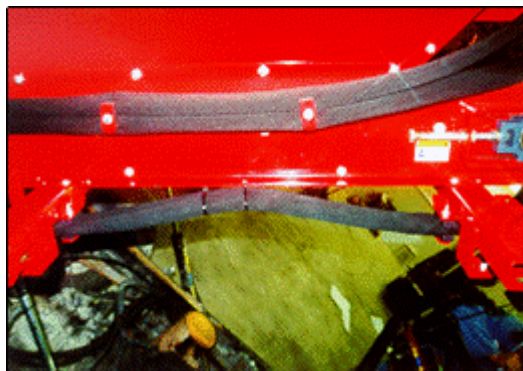
Figure 36: Ensure proper tension of hydraulic hoses
