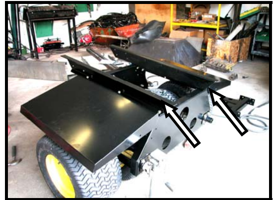
Figure 57: Side Rails Installed
