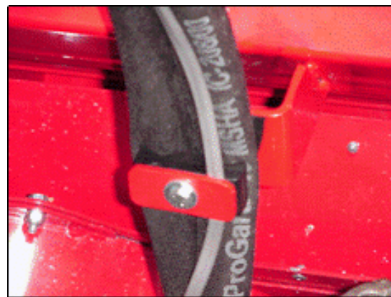
Figure 51: Attaching hydraulic hoses
