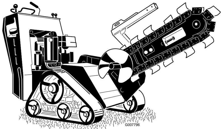
This machine is designed to dig trenches in soil to bury cabling and piping for various applications. It is not intended to cut rock, wood, or any other material other than soil.
