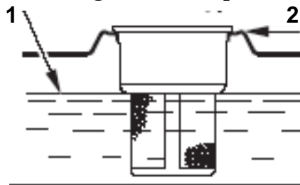
1. Maximum fuel level 2. Fuel tank top
