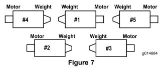
**Note:** Counterweights are shipped installed to the right end of the verticutters. The bolts on the left end are to be used for securing the hydraulic motor.
