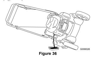
4. **Slowly** pour oil into the oil fill tube, periodically checking the level with the dipstick, until the dipstick indicates that the engine is full as illustrated in Figure 35. **Do not overfill.** (Max. fill: 20 oz. (0.55 l), type: SAE 30W detergent oil with an API service classification of SH, SJ, SL, or higher.)
