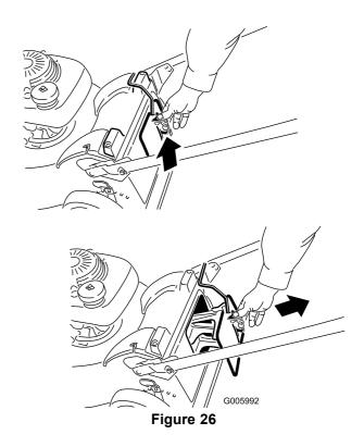
2. Insert the grass bag handle into the grooves at the top of the mower.
