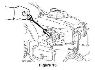
2. Remove the dipstick and check the oil level (Figure 15).
