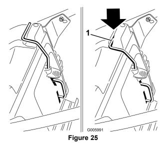
1. Top of recycle plug lever in switch channel
