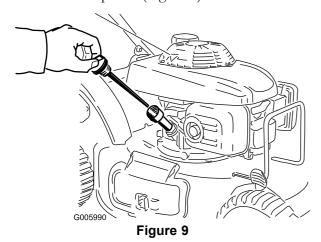
2. **Slowly** pour oil into the oil fill tube, periodically checking the level with the dipstick, until the dipstick indicates that the engine is full as illustrated in Figure 9. **Do not overfill.** (Max. fill: 20 oz. (0.55 l), **type: SAE 30W detergent oil** with an API service classification of SH, SJ, SL, or higher.)
