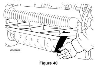
**Note:** Each time the adjusting screw is rotated one click clockwise, the bedknife moves 0.0007 inch (0.0017 cm) closer to the reel. Do not overtighten the adjusting screws.
