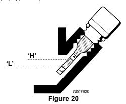
6. Install the oil level gauge and wipe up any spilled oil.
