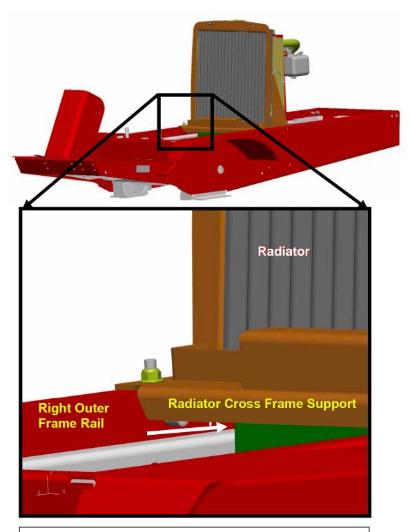
Route Throttle Cable (117-0824) through the opening just below the Radiator support and above the inner right side frame channel (gray colored in this image) back to the engine compartment.
