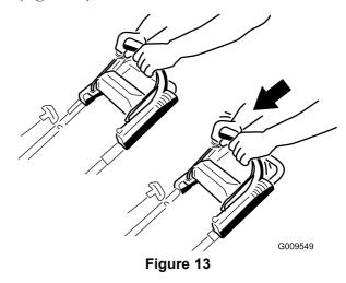
**Note:** If the mower does not freely roll backward after self-propelling, stop walking, hold your hands in place, and allow the mower to roll a couple of inches (centimeters) forward to disengage the wheel drive. You can also try reaching just under the personal pace handle to the metal handle and push the mower forward a couple of inches (centimeters). If the mower still does not roll backward easily, contact an Authorized Service Dealer.
