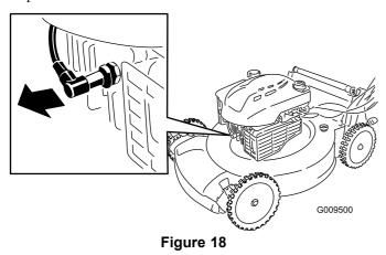
3. After performing the maintenance procedure(s), connect the spark plug wire to the spark plug.
