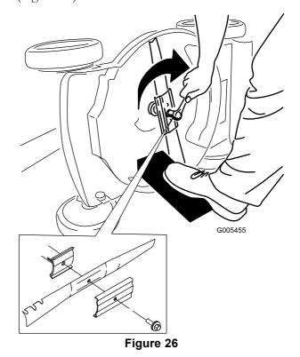
**Important:** Position the curved ends of the blade to point toward the mower housing.
