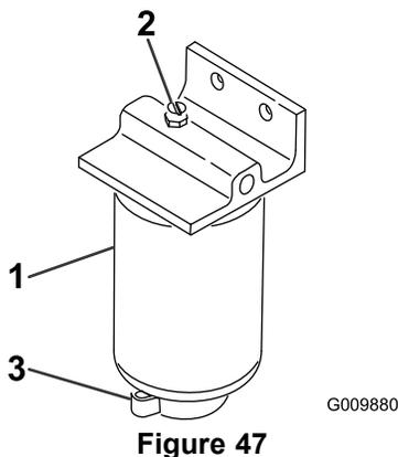
1. Water separator/filter canister
