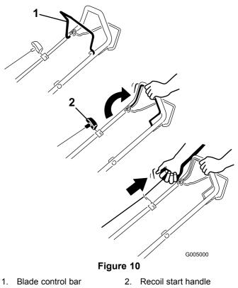
2. Pull the recoil start handle lightly until you feel resistance, then pull it sharply. Allow the rope to return to the handle slowly (Figure 10).
