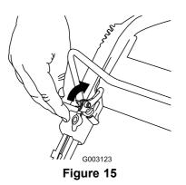
2. Pull the blade control bar to the handle (Figure 16).
