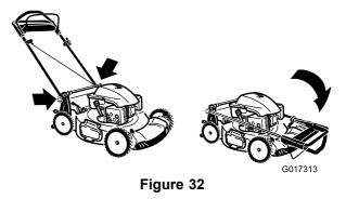
4. To unfold the handle, reverse the steps above.
