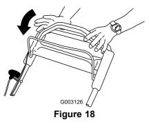
**Important:** When you release the blade control bar, the blade should stop within 3 seconds. If it does not stop properly, stop using your mower immediately and contact an Authorized Service Dealer.
