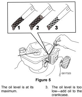
2. The oil level is too high—remove oil from the crankcase.
