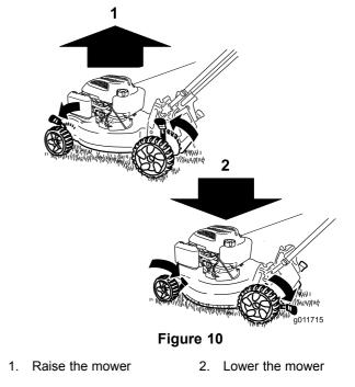
**Note:** The cutting height settings are 1 inch (25 mm); 1-3/8 inches (35 mm); 1-3/4 inches (44 mm); 2-1/8 inches (54 mm); 2-1/2 inches (64 mm); 2-7/8 inches (73 mm); 3-1/4 inches (83 mm); 3-5/8 inches (92 mm); and 4 inches (102 mm).
