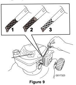
The oil level is at its maximum.  The oil level is too low—add oil to the crankcase.
