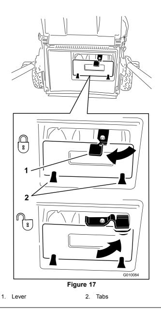
**Note:** To unlock the plug, rotate the lever on the plug to the right (Figure 17).
