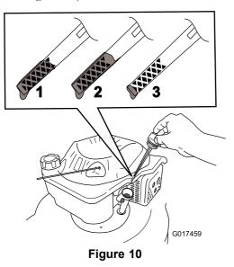
The oil level is at its maximum.  The oil level is too low—add oil to the crankcase.
