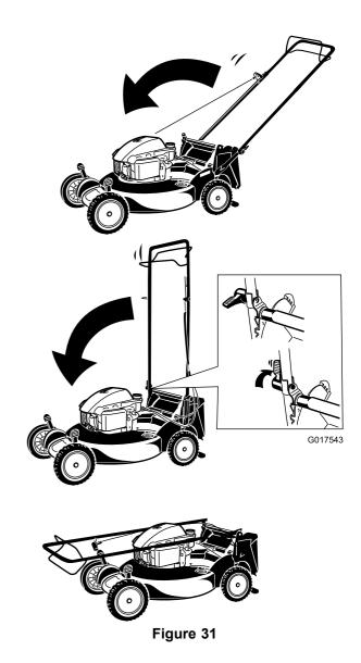
2. To unfold the handle, refer to Assembling and Unfolding the Handle in the Setup section.
