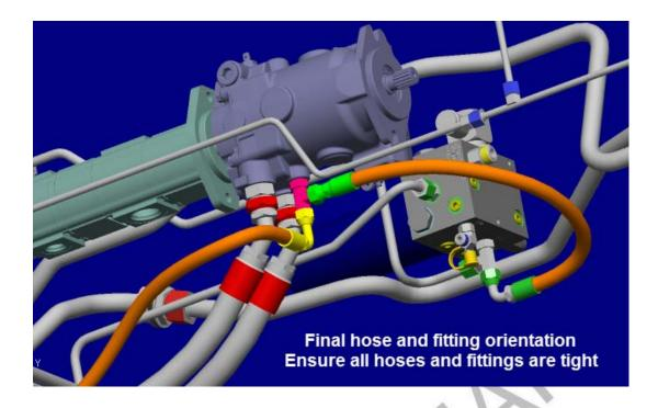
Test-run the unit after the repair to ensure hose-to-deck carrier clearance and check for leaks.
