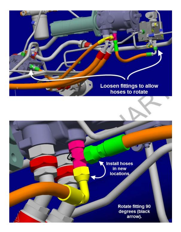
With hoses removed, remove the "T" fitting, replace the seal, reinstall and rotate the hydraulic fitting 90 degree from its original location (pictured in pink with black arrow above). Secure the hose and fitting connections.
