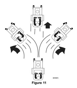
To turn left or right, pull the motion control lever back toward neutral in the desired turn direction. The tines can be in the down position when making gradual turns.
