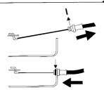
Assemble the grassbag: Identify the grassbag and remove the long ribbon label ( when fitted ) by cutting it off close to the grassbag. Discard the ribbon label.
