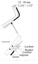
IMPORTANT: Prevent damage - ALWAYS operate the mower with the clutch cable correctly adjusted. ALWAYS replace damaged cables.
