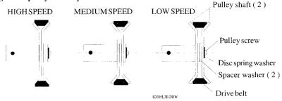
Secure the pulley screw: Tighten to 9 Nm (12lb. ft) torque.
