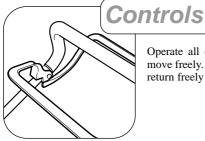
Operate all control levers several times and ensure that the cables move freely. Check that the engine stop and ground drive clutch levers return freely to their rest position when released.
