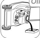
Check the oil level daily before starting the engine and ensure that the correct oil level is maintained. Refer to-'Before Starting the Mower' for oil checking and filling instructions.
