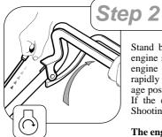
Stand behind the mower and hold the handlebar together with the engine stop lever with your left hand. With your right hand hold the engine start - grip and pull slowly until resistance is felt, then pull rapidly to crank the engine. Carefully return the start grip to the storage position when the engine starts.
