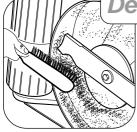
Remove grass debris from the top and underside of the deck housing immediately after use.
