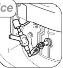
Check the spark plug gap with a feeler gauge and set at 0.76mm.
