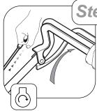
Stand behind the mower and hold the handlebar together with the engine stop lever with your left hand. With your right hand hold the engine start - grip and pull slowly until resistance is felt, then pull rapidly to crank the engine. Carefully return the start grip to the storage position when the engine starts.
