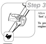
Allow the engine to warm up and move the throttle lever to the **4 fast** position after starting a cold engine.
