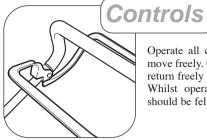
Operate all control levers several times and ensure that the cables move freely. Check that the engine stop and ground drive clutch levers return freely to their rest position when released.
