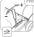
Move the height of cut lever sideways to disengage it from the locking notch, then push forwards to lower or pull backwards to raise the height of cut. Release the lever in the required position and ensure that it locks firmly into one of the seven notch settings.
