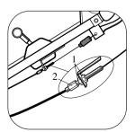
Unscrew the lock nuts (1) and screw the adjuster (2) in or out as necessary. Tighten the locknuts (1) when correctly adjusted.
