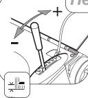
Move the height of cut lever sideways to disengage it from the locking notch, then push forwards to lower or pull backwards to raise the height of cut. Release the lever in the required position and ensure that it locks firmly into one of the seven notch settings.
