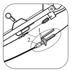
Unscrew the lock nuts (1) and screw the adjuster (2) in or out as necessary. Tighten the locknuts (1) when correctly adjusted.
