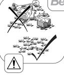
To prevent accidents thoroughly inspect the area and remove all objects which when contacted by the mower cutterblade could become dangerous projectiles. Inspect the area for hidden obstructions which when contacted by the cutterblade could risk health and safety. Remember the location of these obstructions and ensure that you mow around them.
