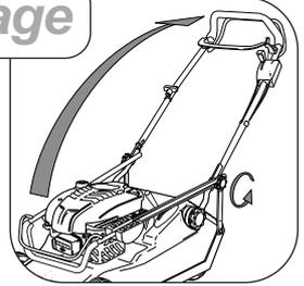
To store the handlebar unscrew the 2 small securing knobs sufficiently to allow it to be pivoted forwards to rest against the mower. Take care to ensure that the control cables do not become snagged at the pivot point and depress the engine stop lever to prevent it being damaged through contact with the engine spark plug.
