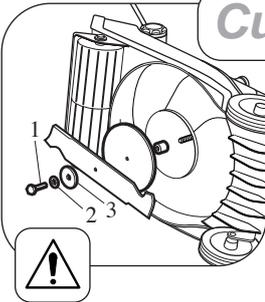
Assemble the cutterblade with the turned up edges facing towards the engine. Secure the cutterblade using the bolt (1), spring washer (2), and distance piece (3) and tighten to a torque of 54Nm
