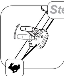
Allow the engine to warm up and move the throttle lever to the 'fast'
