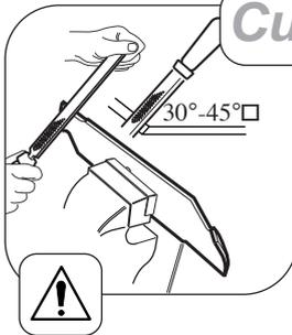
A slightly worn cutterblade may be re-sharpened. Both blade edges must be sharpened equally to ensure balance. Sharpen the cutterblade every 25 mowing hours or more frequently if conditions require. Remove the cutterblade from the mower and clean using a brush and water. Inspect the cutterblade for signs of damage. Sharpen both cutting edges with a flat file to restore performance.
