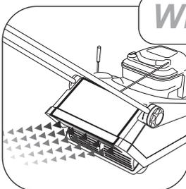
Remove the grassbag and operate the mower with the rear deflector in the closed position.
