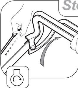
Stand behind the mower and hold the handlebar together with the engine stop lever with your left hand. With your right hand hold the engine start - grip and pull slowly until resistance is felt, then pull rapidly to crank the engine. Carefully return the start grip to the storage position when the engine starts. If the engine does not start after 5 attempts - refer to "Trouble Shooting".
