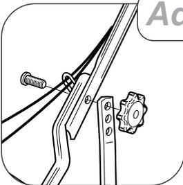
Unscrew the two handlebar securing Knobs to release the handlebar brace then loosen the two nyloc nuts at the base of the handlebar sufficiently to allow it to be moved to the upper, middle or lower position. Re-attach the handlebar brace in relevant hole for best position and comfort. Ensure that both sides are set to the same height. Tighten both the nyloc nuts and knobs to secure the handlebar in place.
