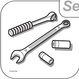
Regularly check that all securing nuts and bolts are tight. Replace missing or damaged items immediately.
