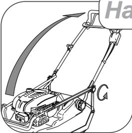
Unscrew the handlebar securing knobs sufficiently to allow the handlebar to pivot. Move the engine stop lever away from the engine to avoid damage and unfold the handlebar to the operating position. Make sure the knobs are assembled to the outside of the handlebar and tighten to secure in position.
