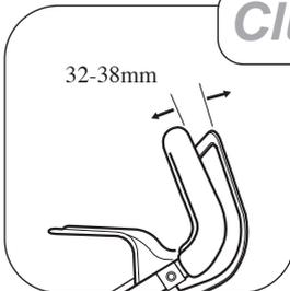
Check the clutch cable operation every 25 operating hours and adjust if necessary. The clutch cable is adjusted correctly when the belt drive just engages with the clutch lever positioned 32-38mm from the handlebar.
