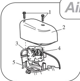
To service the air cleaner, loosen the two screws (1) and remove cover (2). Carefully remove pre-cleaner (3) and cartridge (4) wash in a solution of liquid detergent and water. Allow to air dry thoroughly before fitting.
