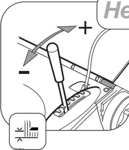
Move the height of cut lever sideways to disengage it from the locking notch, then push forwards to lower or pull backwards to raise the height of cut. Release the lever in the required position and ensure that it locks firmly into one of the seven notch settings.
