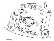
**Grass deflectors:** The rear grass deflectors must always be correctly fitted. The deflectors should be set as low as possible to deflect grass discharge to the ground.
