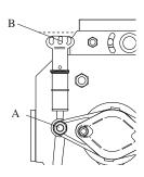
Tighten nut 'A' both ends.
