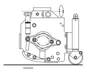
Floating MK3 200mm (8") Cutterheads: When the mower is set up with floating cutterheads the height of cut is gauged by the front and rear rollers. The cutterhead is allowed to pivot fore and aft as well as laterally. This arrangement is recommended for high quality grass areas and performs well where grass is short and the ground undulations are severe.
