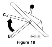
**Note:** This intermediate position (C) is not the normal operating position of the blade control bar. However, it helps to detect a sticking blade brake clutch system early enough to prevent an unsafe condition later.
