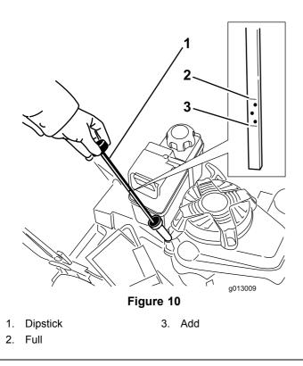
**Note:** When the crankcase is empty, pour about 3/4 of the crankcase capacity of oil in the crankcase, then follow the procedure in this section.
