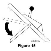
Lift the blade control bar up to about one inch (2.5 cm) below the handle; refer to position A in Figure 16.
