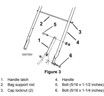
2. Secure the handle latches to the handle with 2 bolts (5/16 x 1-1/2 inches), washers, and locknuts (5/16 x 1-1/2 inches)inch) (Figure 3).
