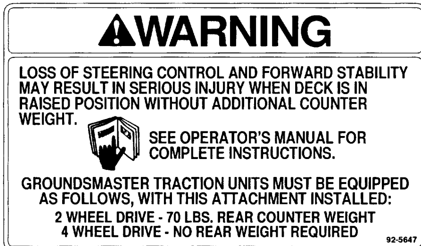
ON FRONT OF CUTTING DECK (Part No. 92-5647)
