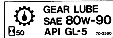
ON ACCESS PANEL & FUEL TANK SUPPORT (MODEL 30455 ONLY), ALSO ON CUTTING DECK GEAR BOX SUPPORT ( Part No. 70-2560 ) Gear Lube Requirements
