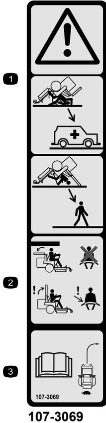
1. Warning—there is no rollover protection when the roll bar is down.
