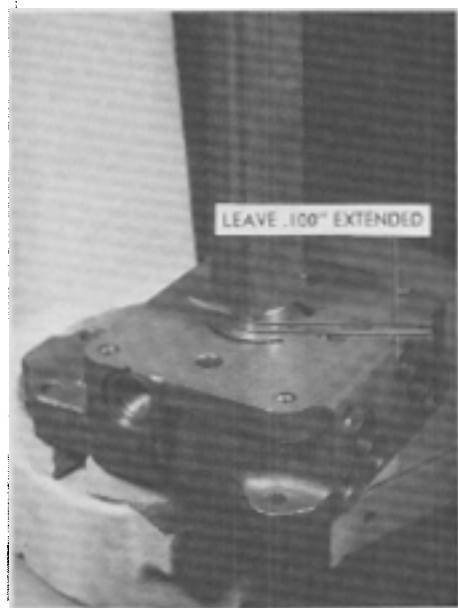
FIG. 82. Install second Needle Bearing
