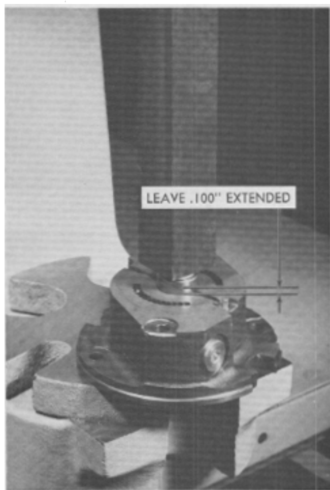
FIG. 54. Needle Bearing Installation
