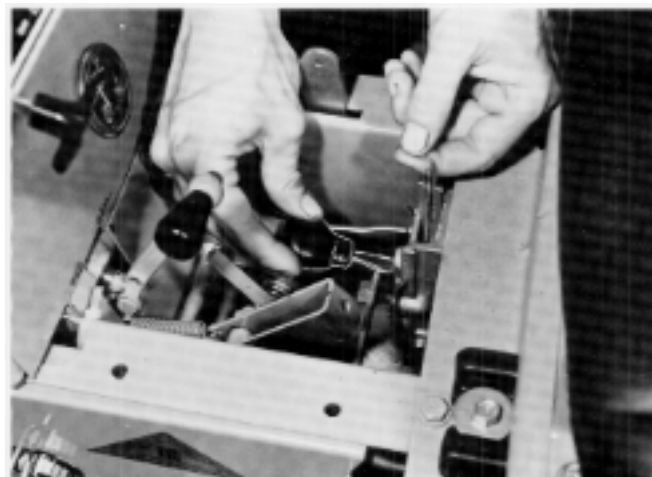
Fig. 5-12 C-Series Automatic, Motion Control Neutral Adjustment
