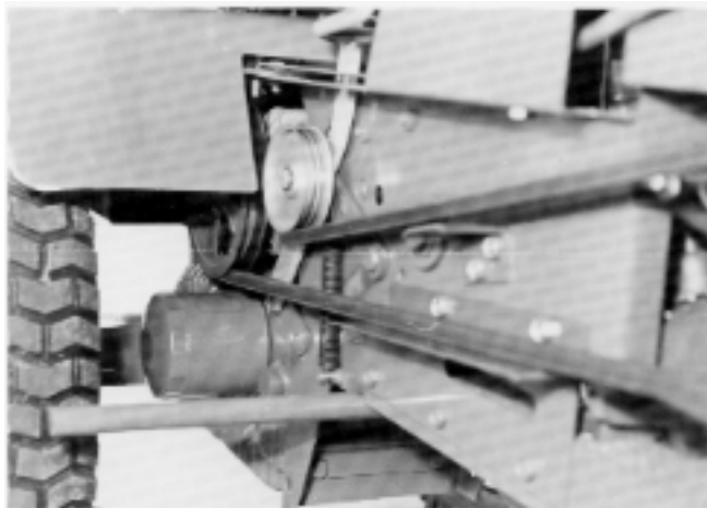
Fig. 5-10 C-Series Automatic, Belt Routing
