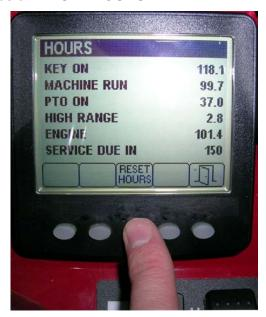
5. Select the HOURS for the appropriate next service time and press the button below the right arrow. A check mark will appear once it has been reset. When finished, press the button below the exit icon (picture of a door open) to return to the main screen, or press cancel to exit.
