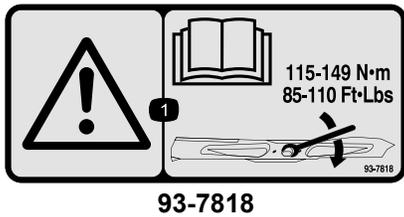
1. Warning—read the *Operator's Manual* for instructions on torquing the blade bolt/nut to 115-149 N-m (85-110 ft-lb).
