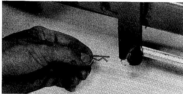
**FIG. 15 Attach Blade Control Rod to Index Handle**
