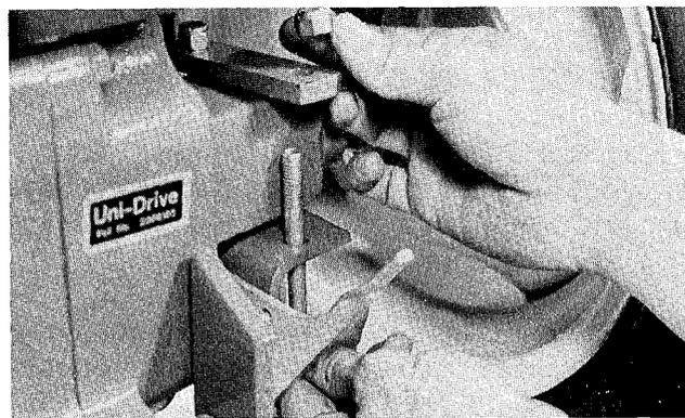
**FIG. 8 Install Two 3/8-16 x 3 3/4 Carriage Bolts & Nuts**
