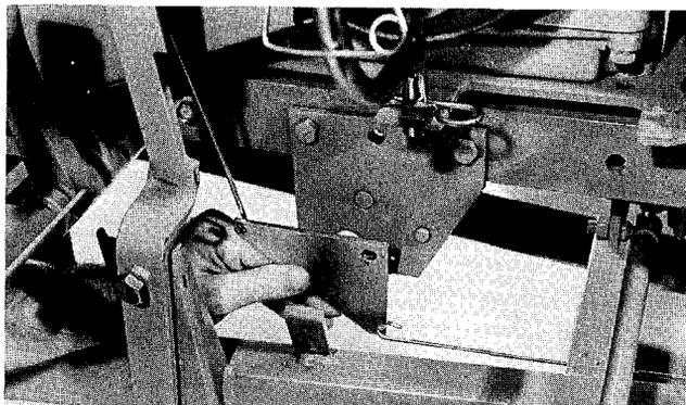
**FIG. 16 Connect Release Rods to Index Plate**
