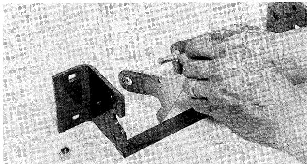
**FIG. 5 Attach Latching Plates to Mounting Bracket**
