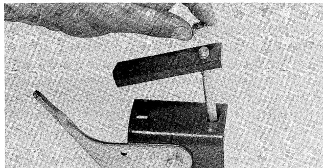
**FIG. 6 Install Metal Links**
