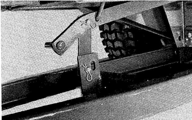
**FIG. 10 Attach Lift Link -1973 and Later Models**
